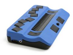
Up to four devices can be connected simultaneously to the Actilino: up to three Bluetooth devices and one USB.
